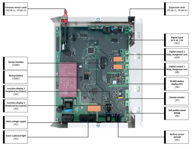
Pressure sensor cards (MC10-1, MC10-2) The pressure sensor cards from SCHNEIDER can be plugged in at will
